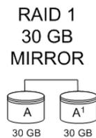
**Figure 2. RAID 1 Configuration Example**
